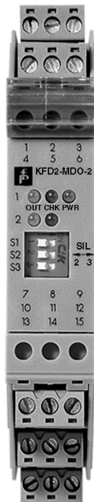
Terminal assignment of field monitor KFD2-MDO-2
